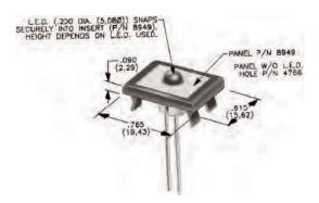
Panel Insert with Hole for LED **Part No.** 894902000
